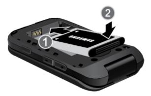
Replace the battery compartment cover, making sure all the tabs are secure and there are no gaps around the cover.
